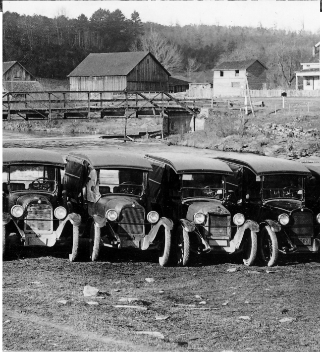
These trucks, with their canvas sides and "new-fangled" pneumatic tires, were "state of the art" vehicles in 1923.
